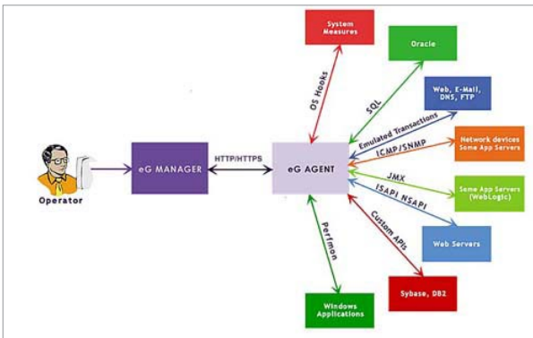
Figure 3: eG Enterprise Single Agent Technology A single agent architecture monitors service, application, server and network status and performance via a centralized management console. This accelerates and simplifies root cause analysis for help desk staff and individual support teams.
