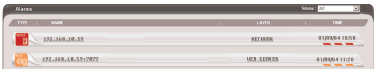
Figure 2: Alarms indicating that the NETWORK layer problem is of a higher priority than the WEB_SERVER problem
