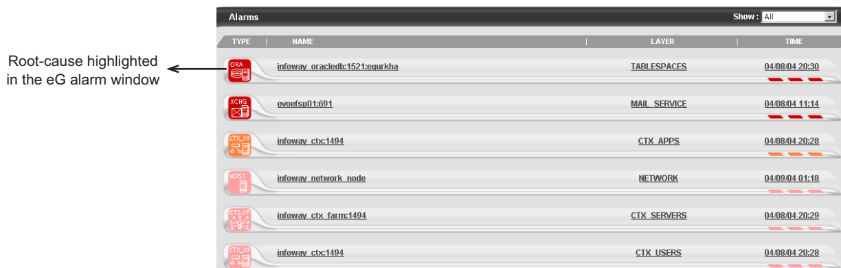
Figure 8c: eG's alarm window showing automatic prioritization of alerts
