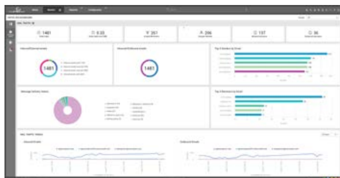
Built-in O365 monitoring dashboards in eG Enterprise v7
