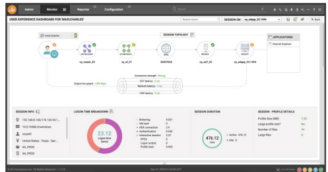
Figure 9: Help desk staff can search by user name and zoom into a specific user's session and analyze latencies they are seeing and resources they are using.
