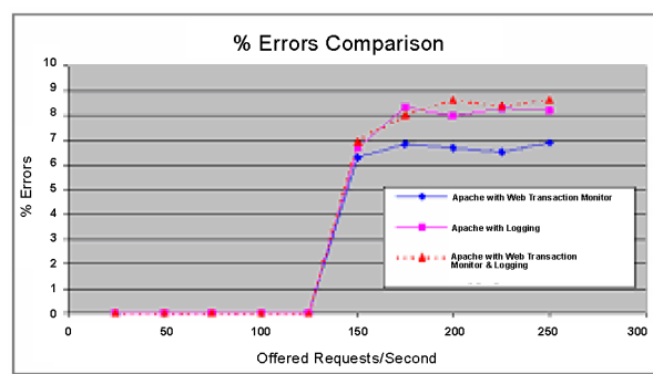
Figure 5 : The performance of an Apache web server as indicated by the percentage of errors generated as the input load is varied for different scenarios
